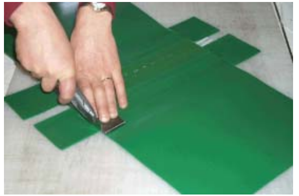
Remove the spacers and cut the belt properly
