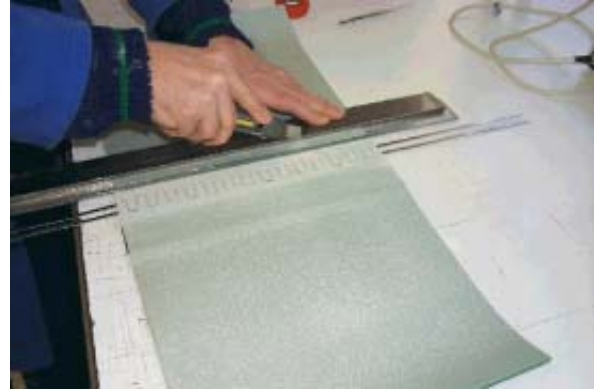
Remove a strip of the lower belt fabric. Use a metal piece to protect the belt below
