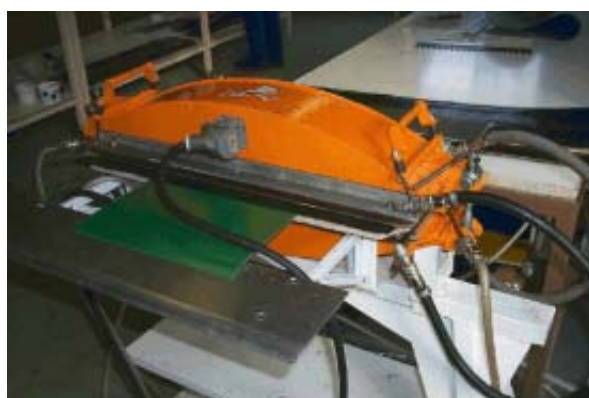
Close the press and start the cooling circuit Follow the instruction of normal belt welding
