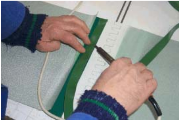
Add a small film to fill the gap and fix it with hot points
