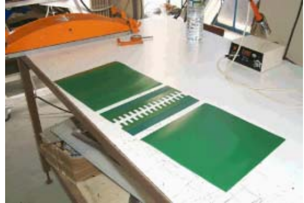
Cutting of the lacing system according to the belt width
