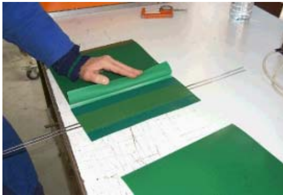
Insert the Lacing system in the belt with 2 pins
