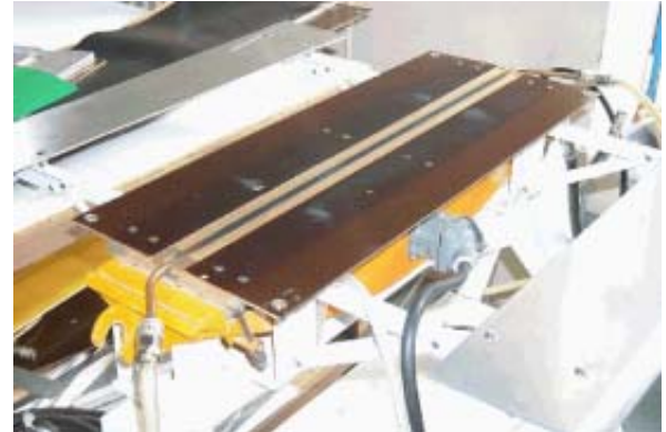
Place the vulcanizing kit in the press
