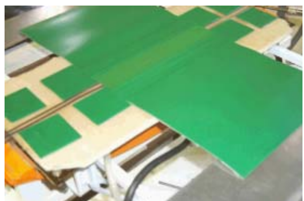
Open the press after cooling. Remove all accessories and the belt
