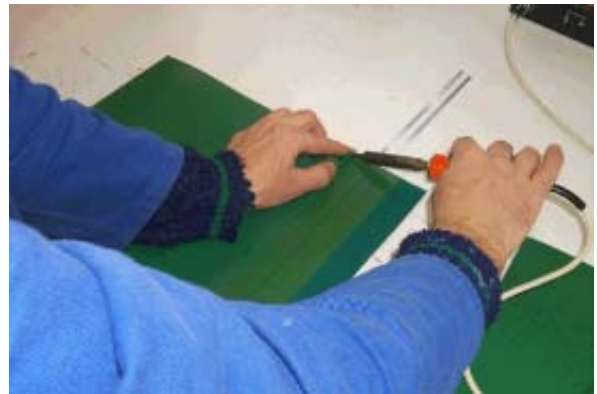
Fix the lacing system with hot points
