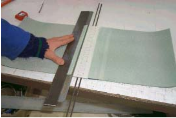
Remove a strip of the lower belt fabric. Use a metal piece to protect the belt below
