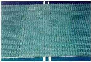
Removable splice without any metal pieces and with approx. the same thickness and color as the belt. No rotation axle, high working tension.
