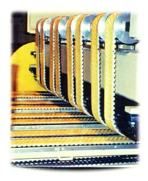
The sheets weigh between 40 to 120 lbs. and they index at 32 feet/min. with an acceleration of 1 G. This machine operates 20 hours/day and 7 days a week.
